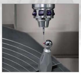
Inspecting and optimizing machine accuracy by calibrating rotary axes with kinematics
