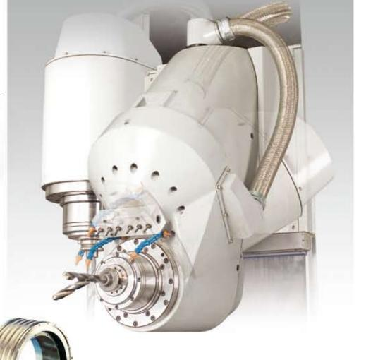
Offers an extra flexibility; the fully automatic 0.001 indexing from vertical to horizontal positions by means of torque motor, this gives operator an extra flexibility: multi-sided machining without re-setting the workpiece; manufacture of complex components with a single set-up; 5 sided machining without additional fixture; 5 axis machining in combination of rotary table.
