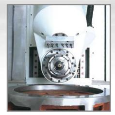
The latest technology torque motor manages the B axis continuous swivel milling head, it guarantees maximum movement dynamic and linearity and thanks to the absence of those traditional mechanical kinematics parts, it results a much higher performance on finishing surface. The direct reading system by a high precision angular encoder is being integrated for
