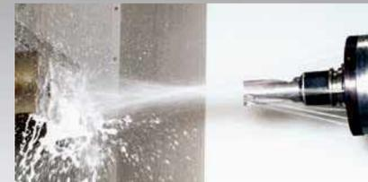
⋮ Coolant through spindle ⋮
