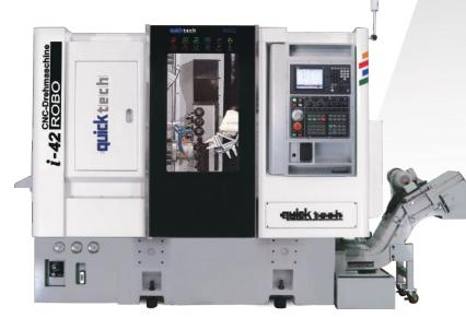
This machine is a modified version of the I-42 with internal integration of a Mitsubishi 6 axis articulated robot. This requires no additional floor space, and is positioned so it will not hinder the machine operator while setting the machine, or operating the Mitsubishi M80 control system. S1(C1)
