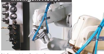
high precision 6 axis robot. This intelligent robot has a total of 88 programs and can easily move around tooling and other obstacles inside the working area.
